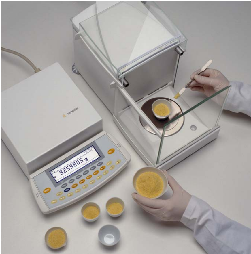
Figure: Sartorius ME36S microbalance with a readability of 1µg and featuring full resolution throughout the entire weighing range up to a 31-g capacity
