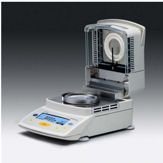
Figs.: Various views of the Sartorius MA150 moisture analyzer
